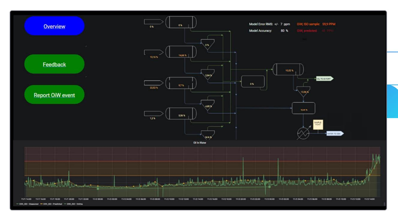
The smart monitoring system displays near real-time data from Cognite Data Fusion®, visualizing it in an intuitive Grafana dashboard. Additionally, calculations combining sensor values and simulator outputs provide engineers with virtual sensors and physical properties they otherwise would not have had readily available.
